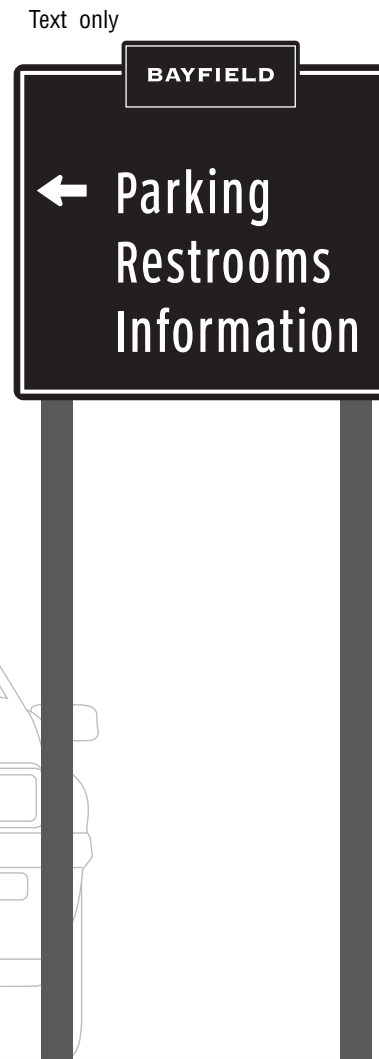
3.1b New Structure 4 x 6" Wood posts with Dk Gray or Black stain
