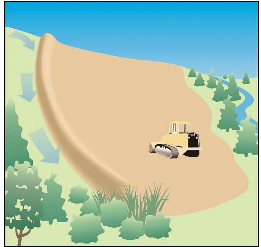
Berms and ditches divert upslope contributing runoff around construction sites and reduce erosion and sedimentation problems. Stabilize berms and ditches after construction.
