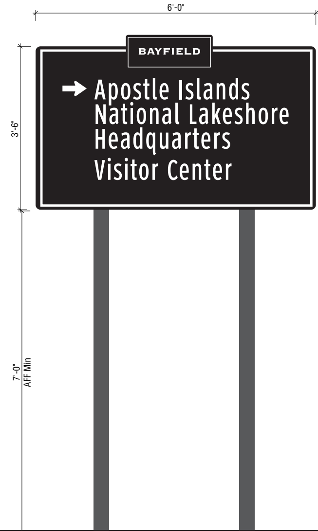
3.1b New Structure 4 x 6" Wood posts with Dk Gray or Black stain
